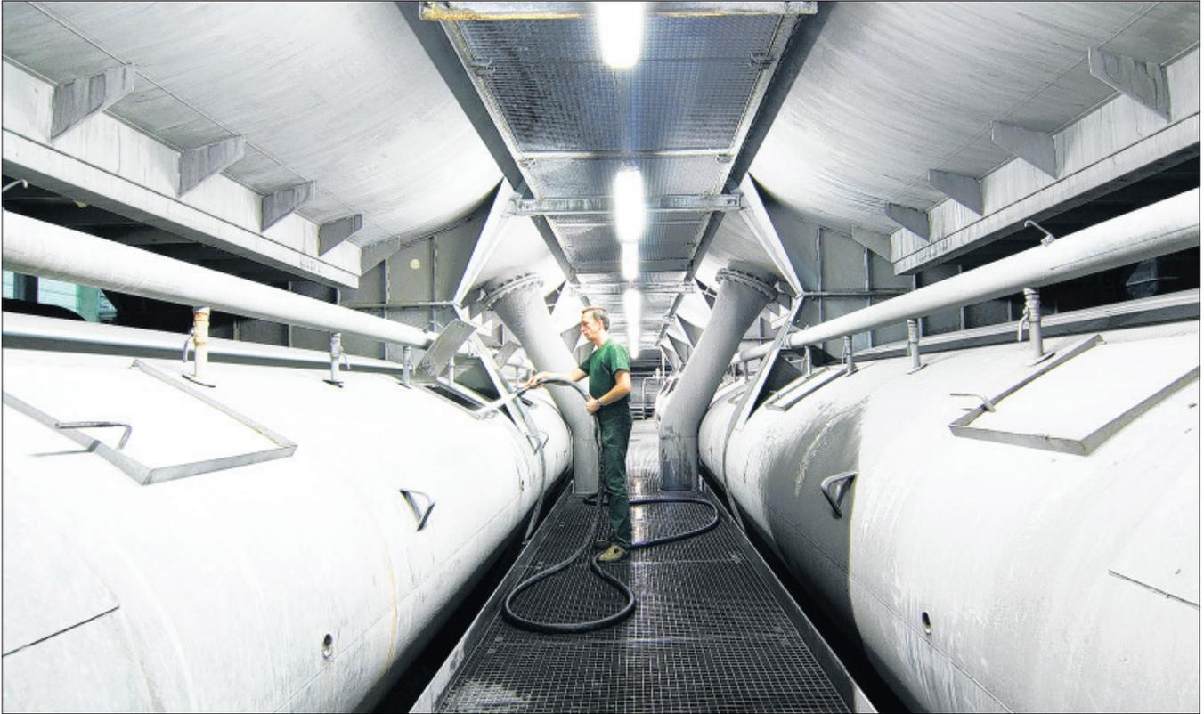
**UPM's deinking plant in Schwedt:** In giant flotation cells the printing ink is removed from the dissolved recovered paper. Foto: UPM
